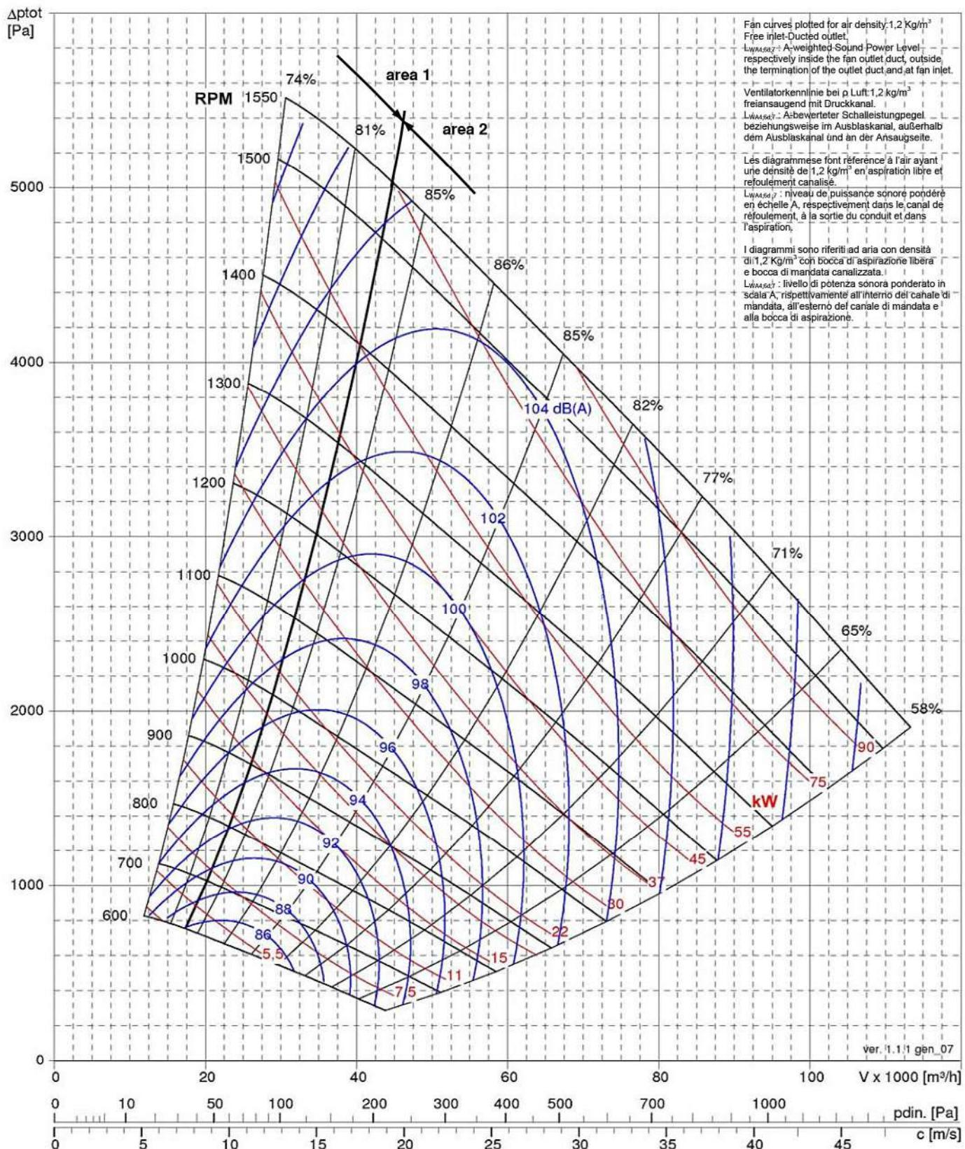
Fan curves plotted for air density 1,2 kg/m<sup>3</sup>
