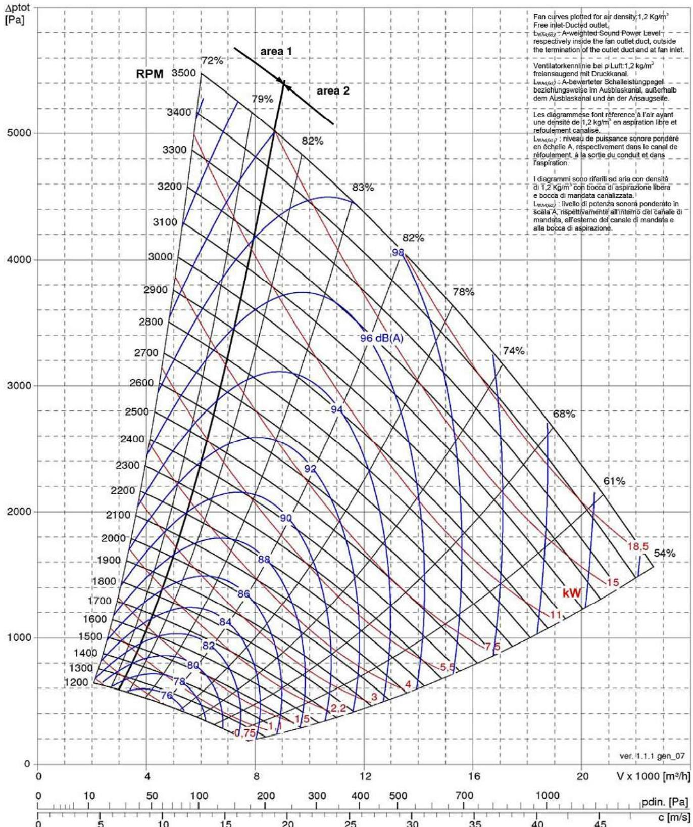
Fan curves plotted for air density 1,2 Kg/m<sup>3</sup>
